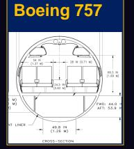
Most Mass and Structure is Below Passenger Floor
